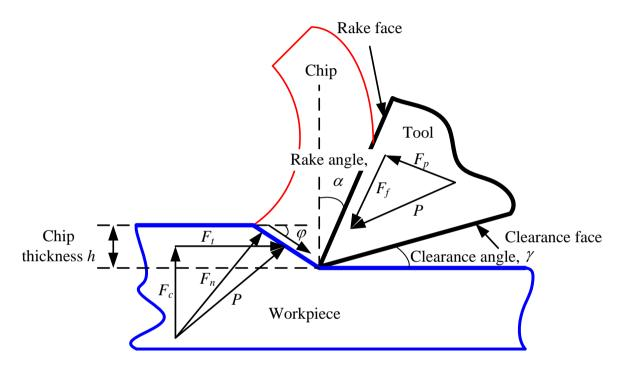
Figure 1. Model of metal cutting by Merchant (1945)
