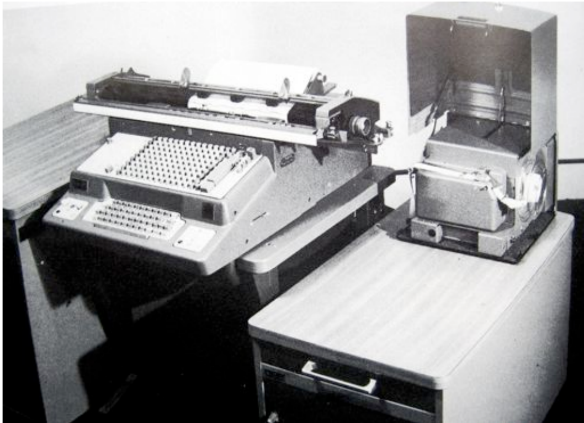
Figure 5. An NCR accounting machine on the left linked to a paper tape punch on the right. Source: P. W. Mace Visible Record Computers (Business Books, 1974), plate 22.
