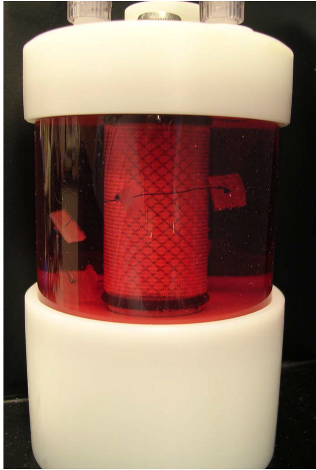
Figure 5 Positioning of PLLA coated scaffolds in the rotating bioreactor. Rotating wall bioreactor flask containing 2% PLLA coated PGA scaffolds, strung on suture to ensure equal submersion and positioning in the rotating flask.
