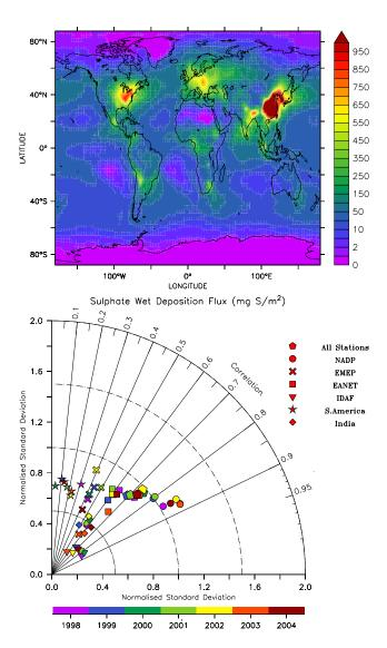
**Fig. 3.** Average annually accumulated wet deposition of sulphate in mg  $S/m^2$  (upper panel) and comparison with observations in a Taylor diagram (lower panel). For the notation see Fig. 2.
