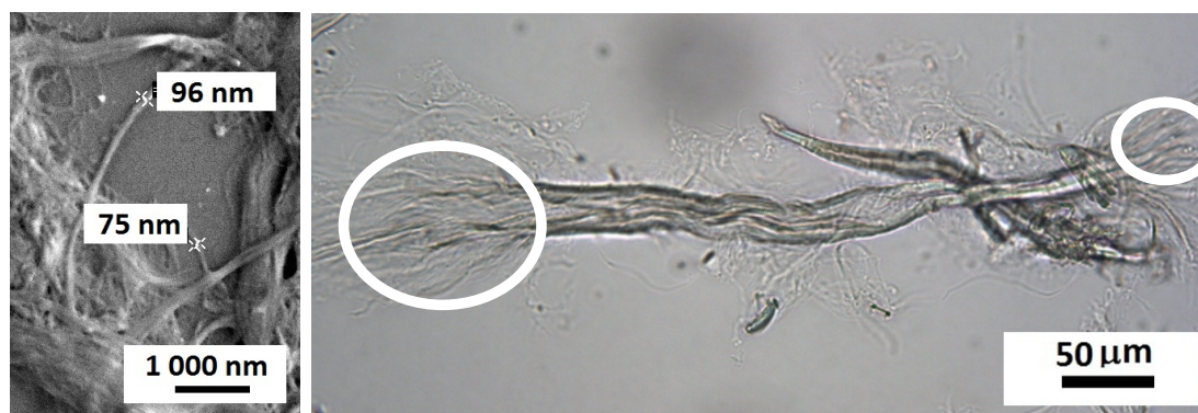
Fig. 4: Nano-CGF amidst pulp produced by synergistic actions of alkaline peroxide and high energy refining. NB: The dimensions given in the picture on the left refer to the fibers marked with white asterisks.
