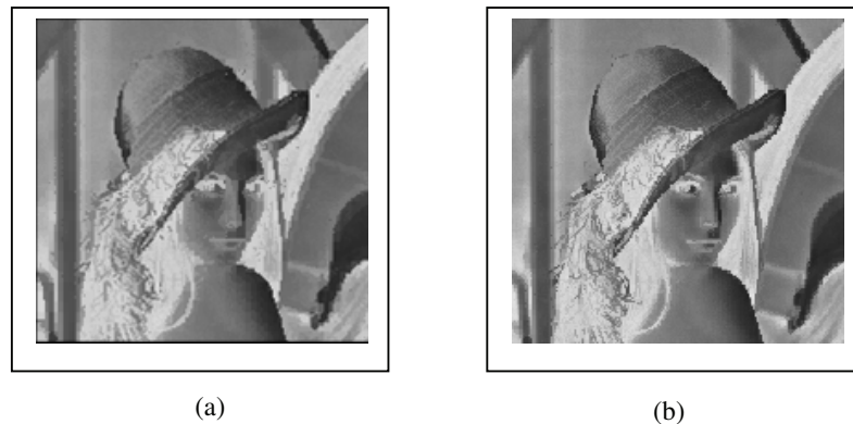
Fig.3. Comparison of the Proposed Work based on Neuro-Statistical Modeling and The Generalized SOM based Image Coder for Lena Image. (a) Generalized SOM method (b) Proposed method
