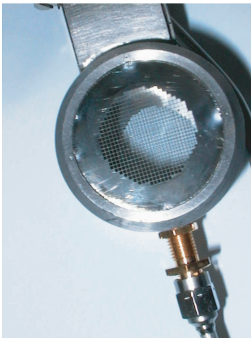
Figure 7: 12.9 GHz cavity used by ASACUSA to measure the hyperfine structure of antiprotonic helium. It has an inner diameter of 28.8 mm, and uses meshes on both top and bottom of the cylinder to let antiprotons and laser beams pass. The microwave radiation is provided by a rectangular wave guide from top, and the magnetic field strength in the cavity is monitored by a pick-up antenna attached below.
