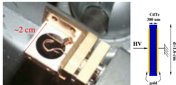
Figure 3. Photo and geometry of the CdTe detector.
