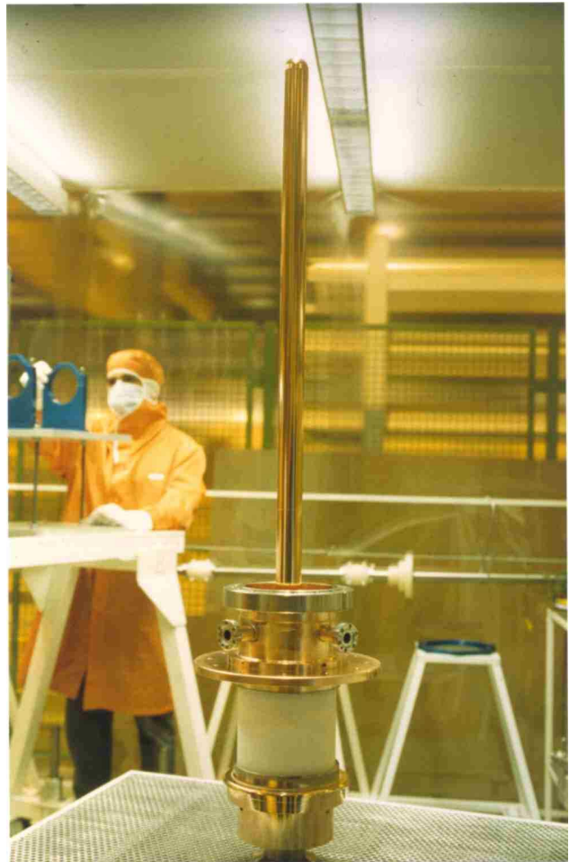
Fig. 5: the 75\Omega fixed couplers. Note the two ports for the vacuum gauge and the electron monitor close to the ceramic.
