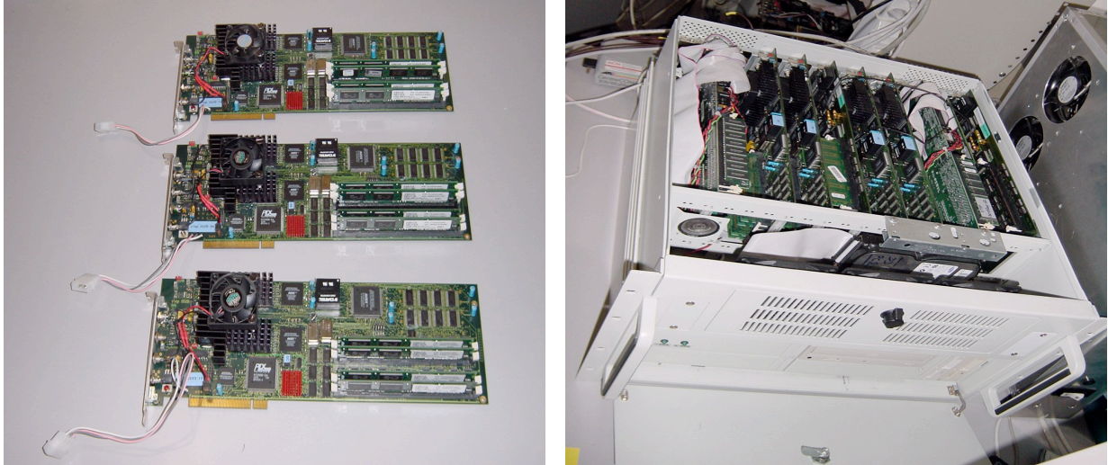
Figure 2.29: The ETEP digitizer modules (left) and the chassis (right).
