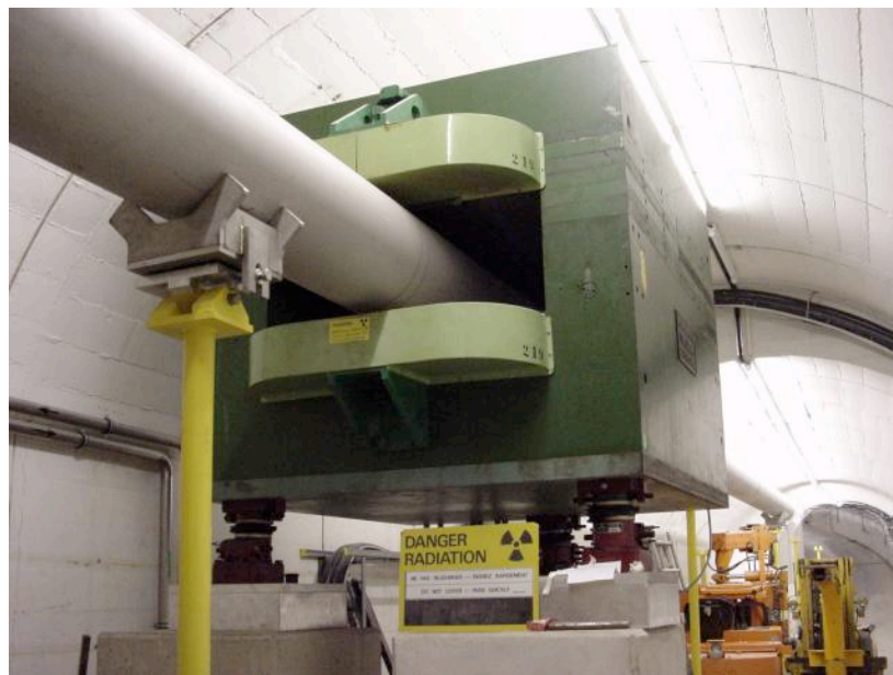
Figure 3.5: The M200-type magnet used as sweeping magnet.
