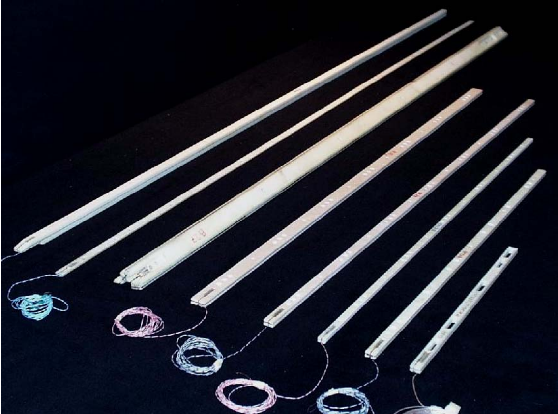
Figure 11. Examples of typical induction coils used for accelerator measurements, by courtesy of J. Billan (CERN). The coils have length ranging from 25 cm to more than 2 m much larger than its extension in the cross section (10 mm to 50 mm), and windings of negligible dimensions with respect to the overall size of the coil (typically 0.5 x 0.5 mm).
