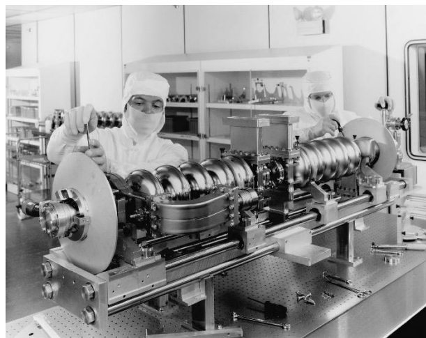
Fig. 1. CEBAF cavity assembly in the clean room.
