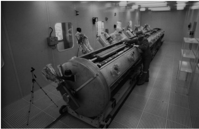
Fig. 2. LEP2 RF module assembly in the clean room.
