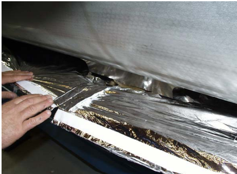
Fig. 11 VELCRO® fasteners for fixing multilayer insulation blankets
