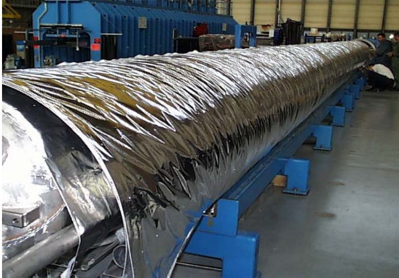
Fig. 10 Prefabricated multilayer insulation blankets upon installation
