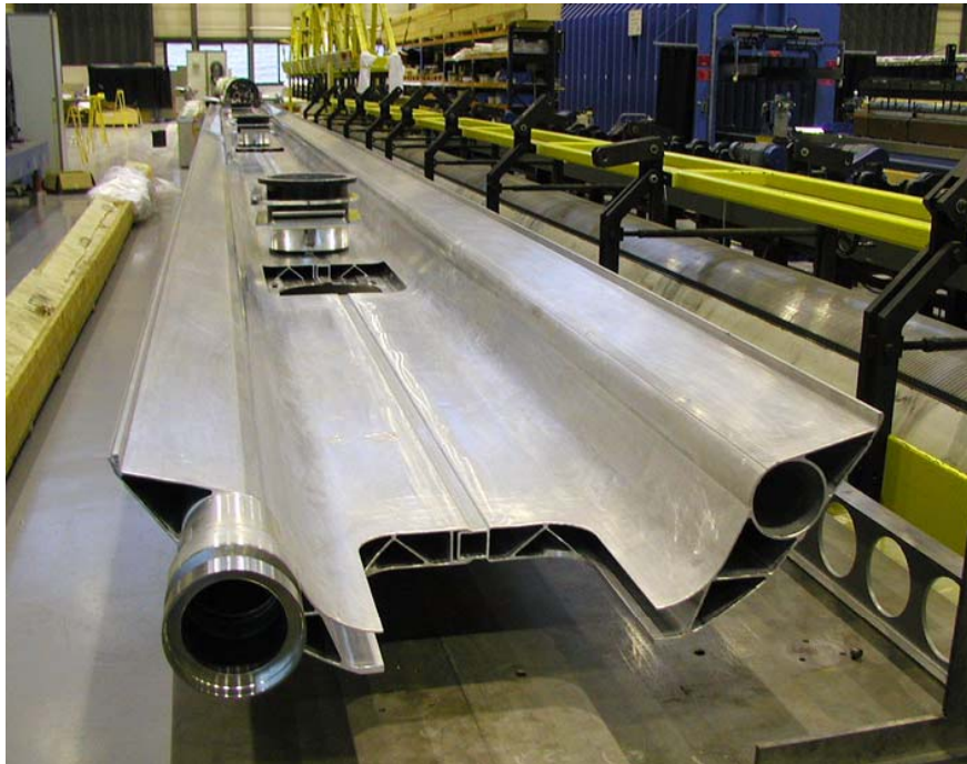
Fig. 8 Thermal shield extruded “bottom tray” with integrated cooling channel
