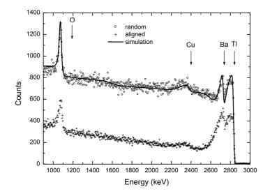
Figure 4 : Helium backscattering spectra of a Tl<sub>1.85</sub>Ba<sub>2</sub>CuO<sub>6</sub>/LaAlO<sub>3</sub> thin film after growth, using random (o) and aligned (+) beam incidence, along with a simulated spectrum (---). The scattering angle of the detected particles is 172°.
