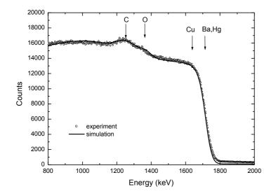
Figure 2 : Proton backscattering spectra of a HgBa<sub>2</sub>CuO<sub>(4+s)</sub> pellet after growth (o) along with a simulated spectrum (----). The scattering angle of the detected particles is nearly 180°.
