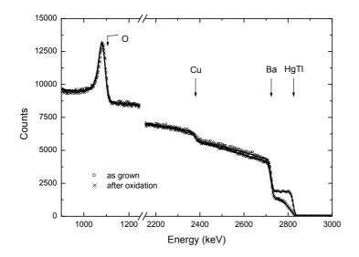
Figure 3 : Helium backscattering spectra of a Hg<sub>x</sub>Tl<sub>1-x</sub>Ba<sub>2</sub>Ca<sub>2</sub>Cu<sub>3</sub>O<sub>(2n+2+s)</sub> pellet after growth
