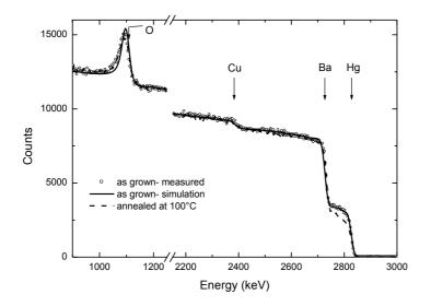
Figure 1 : Helium backscattering spectra of a HgBa<sub>2</sub>CuO<sub>(4+s)</sub>\_pellet after growth (o) along with a simulated spectrum (—), and after vacuum annealing at 300°C (----). The scattering angle of the detected particles is 172°.
