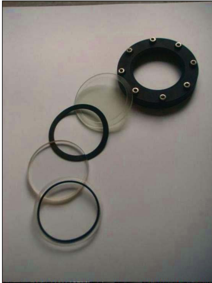
Fig. 3.5: Window's components: port-hole with screws, quartz, Plexiglas and o-rings
