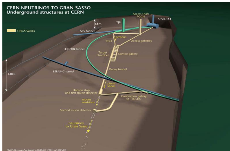
Fig. 1.7: CNGS underground structure
