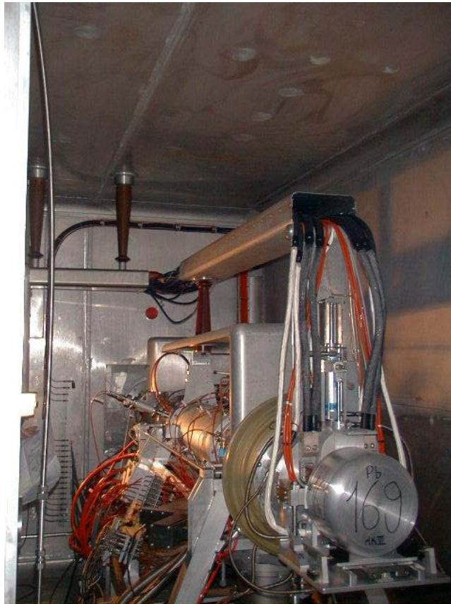
Fig. 3.2: GPS front end with conventional target installed
