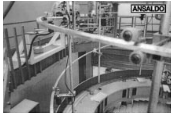
Fig. 6. View of the conductor during transfer inside the winding machine, when winding the first layers of the winding prototype.
