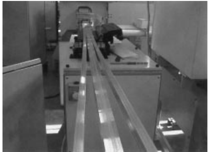
Fig. 2. View of the insert and the two reinforcements sections entering into the EB welding unit at a feed speed of 2 m/min.
