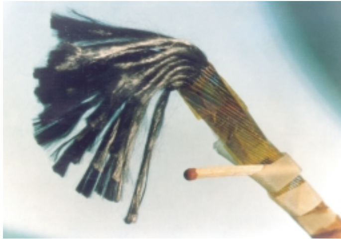
Fig. 3: HERA's superconducting cable is made up of 24 wires, 1230 filaments each, with a diameter of 14 microns
