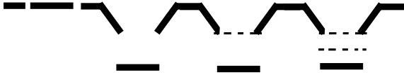
FIG. 6: An array of collectors is shown; from left to right is (a) a flush collector, (b) a recessed collector or capacitive probe, (c) a 1-grid, and (d) a 2-grid collector.
