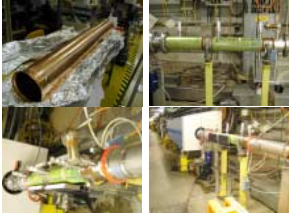
Figure 3: Photographs of the WAMPAC copper screen and of WAMPAC installed in the SPS section 417 with and without dipole magnets.
