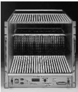
Fig. 5-25. Picture of the F6859 CERN crate. The upper rear half is free.
