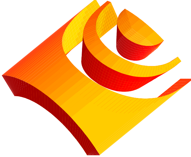
Fig. 7: Artists view of the endspacers for the quadrupole, outer layer coil
