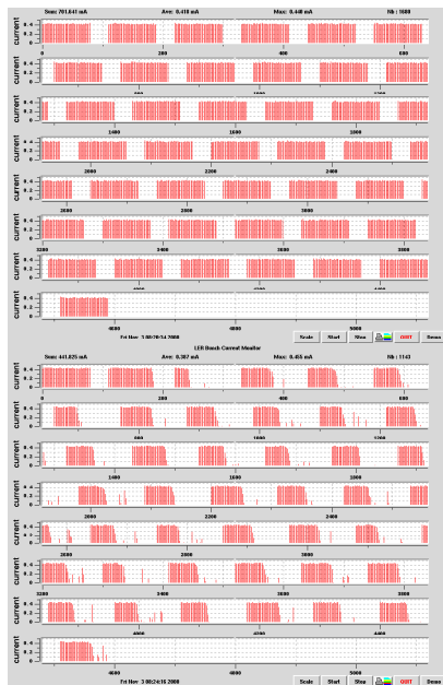
Figure 4: Special filling pattern before (upper) and after (lower) switching off/on the feedback.
