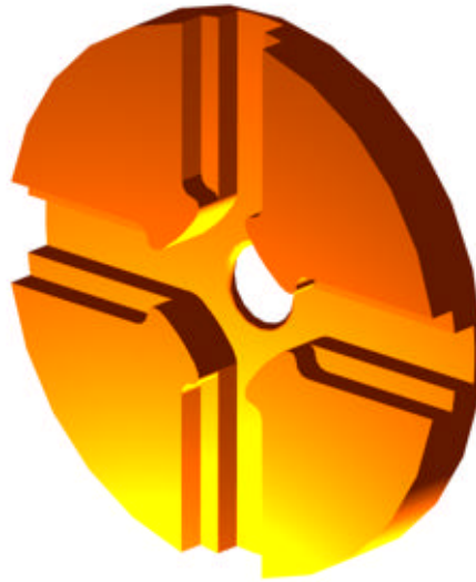
FIGURE 5. Low surface electric and magnetic field geometry, XDS. The low surface electric field is accomplished through a thick iris with an elliptical cross section. The low surface magnetic field is accomplished through the profiled convex outer cavity walls, in distinction to the usual, turned, concave outer cavity wall.
