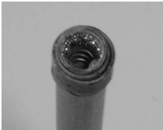
Figure 3: Tip of the micro-oven, showing droplets of indium.
