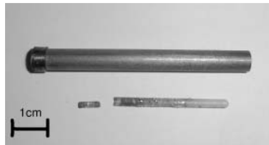
Figure 4: The oven and the alumina sample tube. The small piece is a molybdenum plug to close the sample tube partially.
