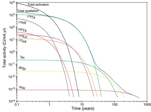
Figure 12: Evolution of the radioactivity (Ci/mA·yr) of the tungsten spallation target as a function of time.
