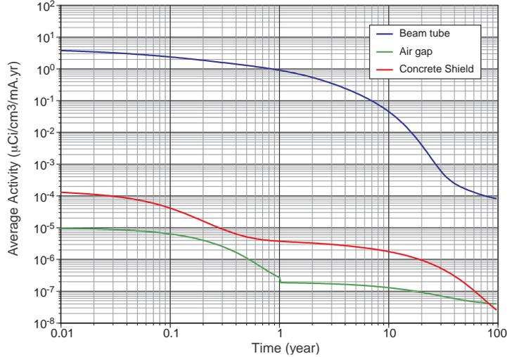
Figure 14: Evaluation of the radioactivity from the beam line due to normal beam losses (1 nA/m of beam losses along 10 m of straight section.)
