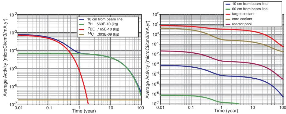
Figure 13: *Left*: Evolution of the radioactivity of water 10 cm from the beam line due to normal beam losses (1 nA/m of beam losses along 6 m of straight section). *Right*: Evolution of the radioactivity of water coolant in different parts of the reactor core.
