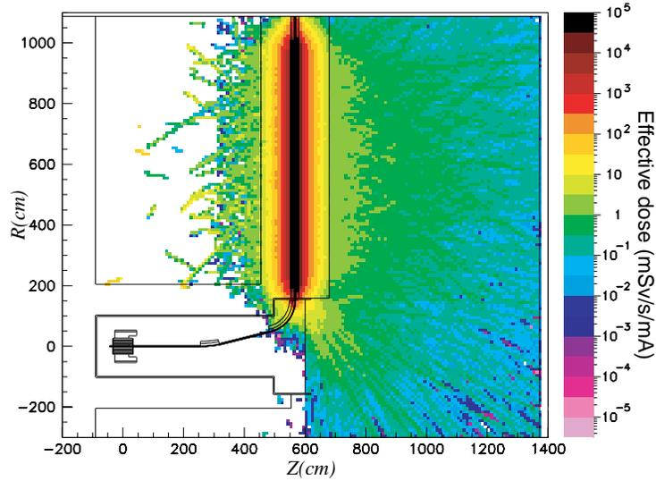
Figure 6: Estimation of the particle dose rate to human body escaping the beam transfer line per mA of beam losses, in the shielding configuration with 1 m thick barytes concrete.
