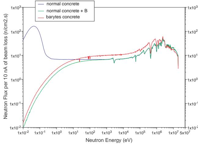
Figure 7: Neutron flux spectra for different compositions of the concrete shielding (1.4 m thick) per 10 nA of beam loss.
