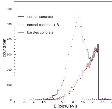
Figure 8: Spallation neutron spectra in the shielding for different concrete compositions. As expected, the spectra are sensitive to the presence of barium. See explanation in the text.
