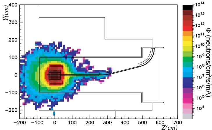
Figure 2: Neutron flux distribution ( $\text{n/cm}^2/\text{s/mA}$ ) following the impact of the proton beam on a solid tungsten target in the TRADE experiment.
