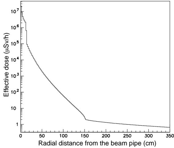
Figure 11: Effective dose as a function of the radial distance to the beam pipe for a beam current of 0.25 mA and  $10^{-6}/\text{m}$  beam losses for the reference shielding configuration.
