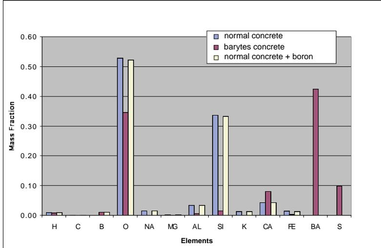
Figure 4: Chemical composition of the three different concrete materials used (in weight fraction).
