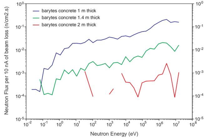
Figure 5: Variation of the neutron flux spectra escaping the beam transfer line as a function of the thickness of the concrete shield.
