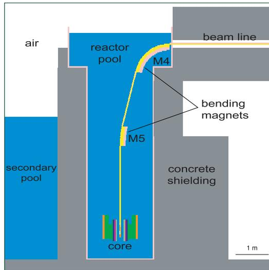
Figure 1: View of the geometry of the TRADE experiment as implemented in the FLUKA calculations.
