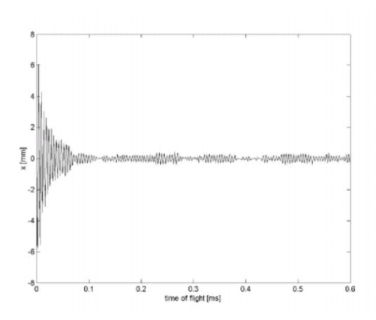
Figure 1: Simulated displacement from an optical axis as a function of time-of-flight
