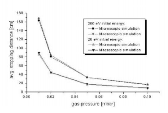
**Figure 2:** Cooling length as a function of pressure of buffer gas (He) for the ions with mass A=100 in room temperature.
