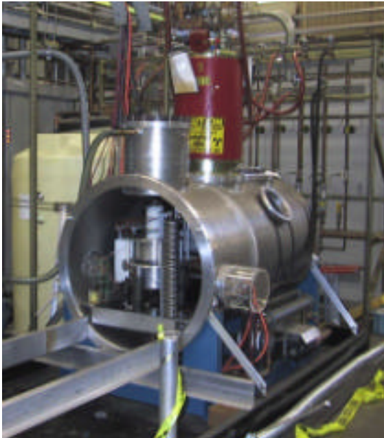
Figure 1. Left: Modulator Tank w/ 5045 klystron, Right: Multi-lam pins for ground
