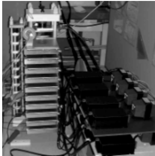
Fig. 5 View of the IGCT switch during pre-testing on the manufacturer's site.
