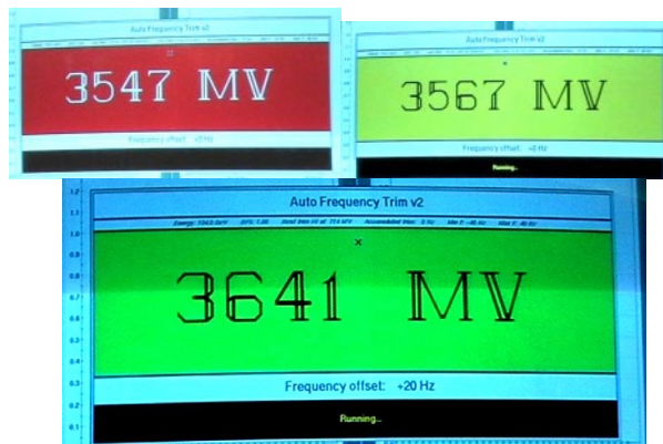
Figure 7: Display output (total RF voltage) of the computer program that automatically controlled J_x . The three cases correspond to 1 klystron off (upper left), recovering (upper right), and all normal (bottom).
