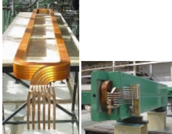
Figure 2: First MSIB coil (left), preseries magnets MSIB01 (top) and MSDC01 (bottom)
