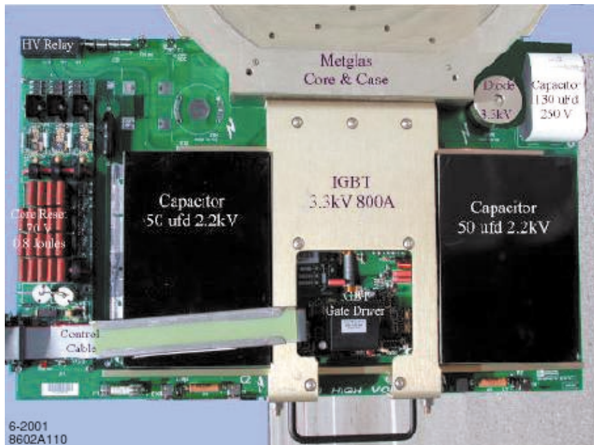
Figure 4.7: Induction cell driver board.
