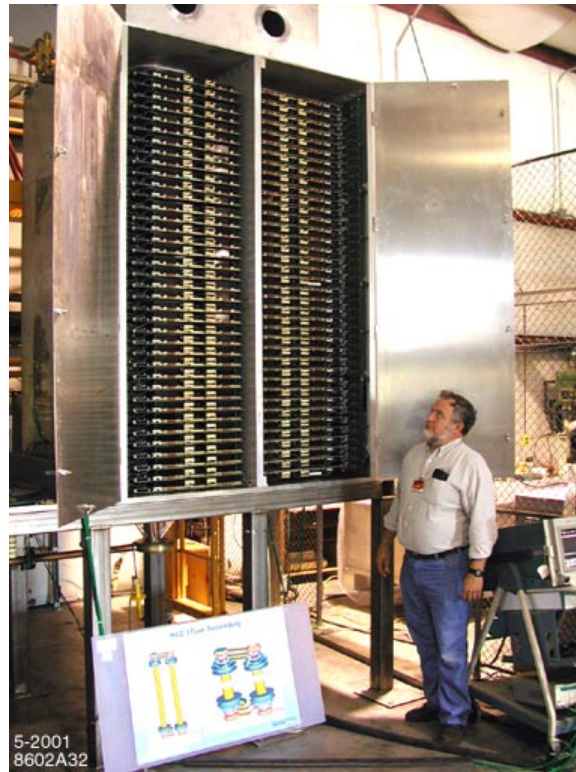
Figure 4.11: Full-scale modulator prototype with drivers installed.
