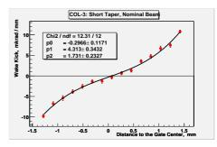
Figure 1: Deflection angle versus beam-to-collimator offset for collimator 3.
