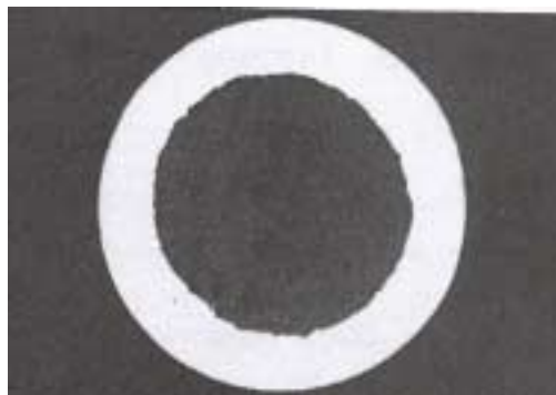
Figure 2-10. Cross-section of monofilamentary BSCCO 2212 wire.
