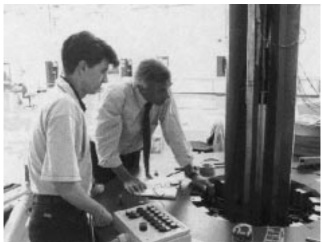
Fig. 3. New collaring press operating for first mock-up test in fabrication hall. A hole in the ground provides the vertical passage of the collared coils.
