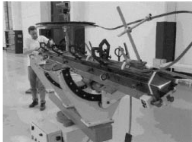
Fig. 2. Coil winding machine in operation.
