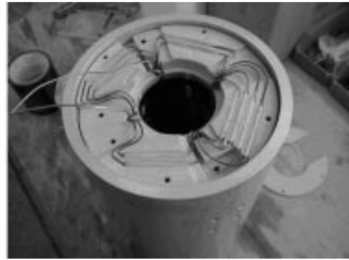
Fig. 3. MQTB electrical connections. Not only must the 4 coils be connected in series, but also the 6 layers in each coil.
