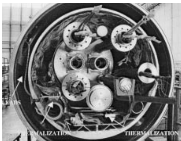
Fig. 5. Prototype 60 A leads integrated in SSS3.
