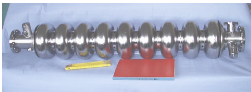
Figure 1: The 9-cell Niobium cavity for TESLA.
