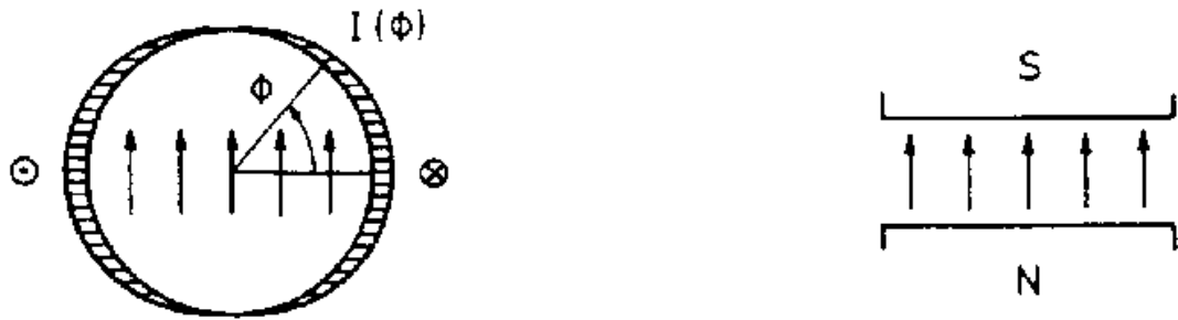
Figure 5.1: Generation of a pure dipole field by a \cos(\phi) current distribution and positive ( \otimes ) and negative ( \odot ) current densities respectively. The right side shows a conventional dipole magnet with iron pole shoes [59].
