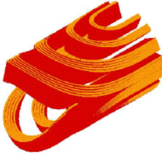
Figure 3.5: The picture shows the coil end of the inner layer of a LHC dipole magnet. The magnetic field in the end section perpendicular to the cable is much lower than in the straight part and can even be zero.
