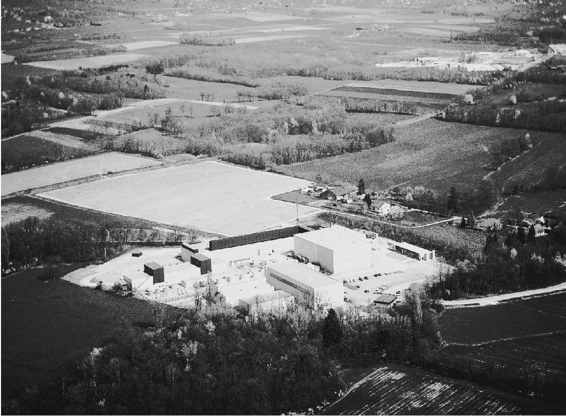
Fig. 4.10: An aerial view of the L3 site. The main building towards the middle of the picture is situated about 40 m above the detector.
