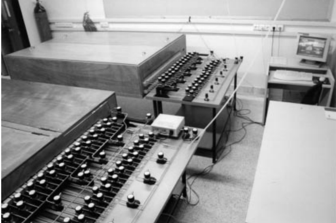
Figure 2. A view of the two Temperature Stabilization Boxes, (TSB) and the respective valve manifold complex. Each valve socket is connected with the corresponding tube (MDT) inside the box via a flexible thinner stainless steel tube.
