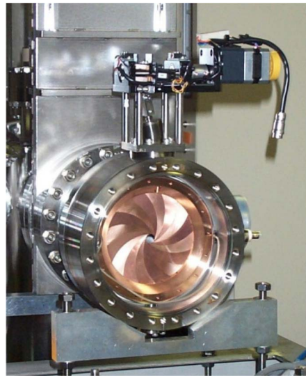
Figure 16: A photo of the variable aperture, which allows high transport efficiency of antiprotons keeping the differential pumping of more than 6 orders of magnitudes.
