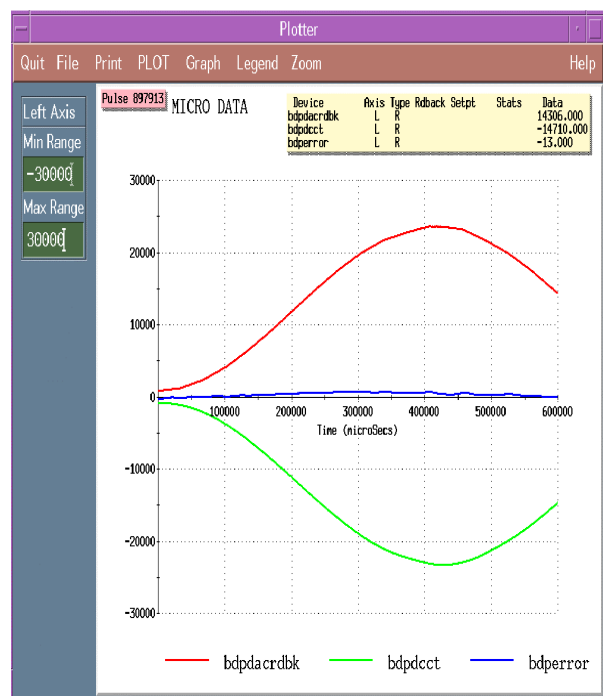
Figure 1: Booster Dipole Signals for one Booster Cycle.
