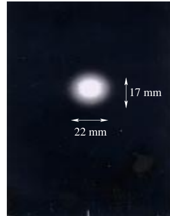
Figure 6.6: Photo of the beam. The horizontal beam-dimensions are 6\sigma=22 mm. The vertical one is 6\sigma=17 mm.
