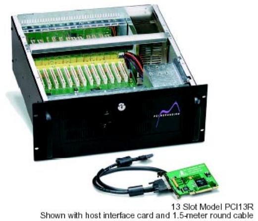
Fig. 10 A PCI cage with 13 slots
