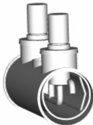
FIGURE 4. The Helium Pump Cryostat. Accessibility for the change of a pump is from the side flanges.
