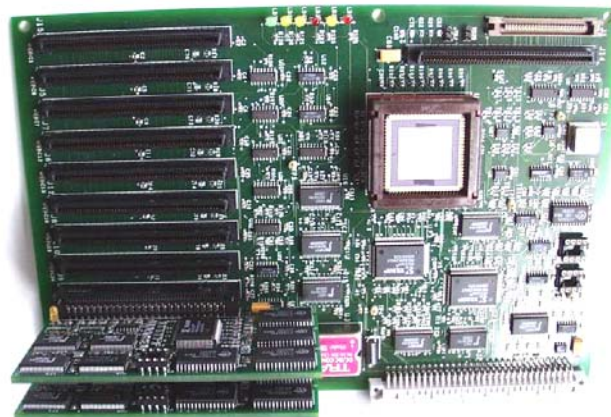
Figure 1: MCC exerciser board with two mounted memory cards.
