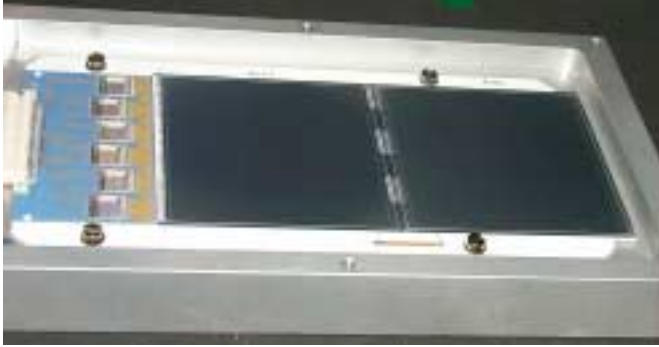
Figure 10: Photograph of 6chip, 12.8cm strip silicon detector (ATLAS type) module.
