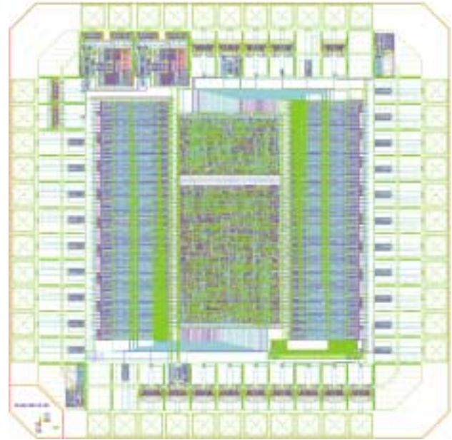
Figure 10: Layout of the BeetleSR 1.0 test chip. The two register blocks are located on the right and left hand side of the chip. The I 2 C interfaces are the blocks in the centre, the SEU robust one being the larger block.
