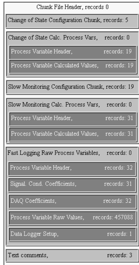
Figure 3: Quench file structure.
